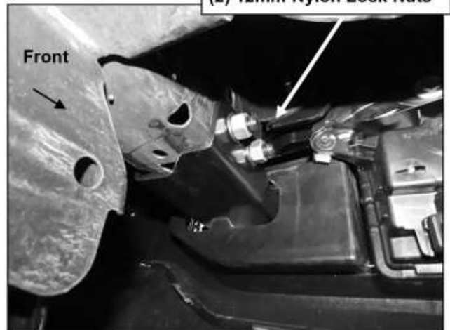
(Fig 8) Outer passenger/right side Bracket with Double Bolt Plate pictured from behind bumper
