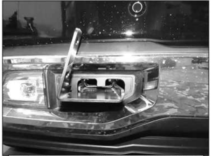
(Fig 11) Passenger/right side Bracket installed
