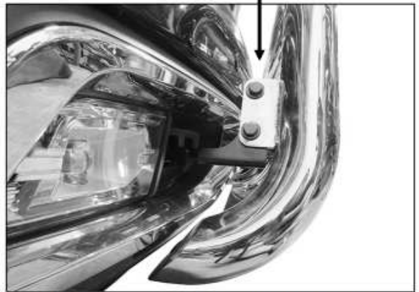
(Fig 13) Passenger/right side complete installation
